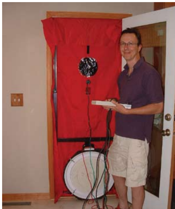
Charlie Richardson uses a blower door during a REAP audit to identify problems such as those found in Chris Hansen's house.
