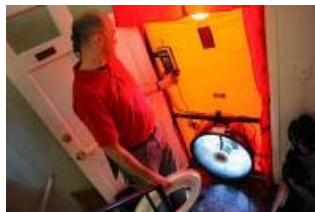
Energy auditor Shawn Le Mons uses a reverse-fan, which simulates wind, and an infrared monitor to detect temperature differentials that indicate leaks in a home. He'll also inspect appliances. (John Leyba, The Denver Post)
